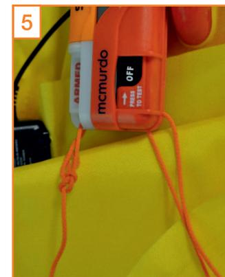
**Attaching the lanyard.** Using the remains of the orange lanyard (which is secured to the bottom of the lifejacket) tie loose end onto the white section of the S20 with a bowline. Ensure that there is plenty of slack in the line so the S20 is not pulled off the oral tube when the lifejacket is inflated. The purpose of this line is purely as a back-up in case the S20 is dislodged from the oral tube.
