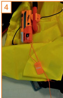
**Folding the Chamber.** Fold the base of the inflation chamber up towards the S20. Tie the orange lanyard using 3 half hitches around the webbing where the inflation chamber is attached to the cover. Tie off as short as possible, taking up all the slack without distorting the shape of the lifejacket.
