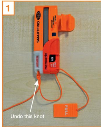
**Untie lanyard.** The S20 is supplied with an orange lanyard loosely tied onto the white section of the S20. Undo this knot, so there is a short lanyard to the orange tab and a long loose lanyard. Slide off the orange arming tab. (Lift the right side slightly & push left with your finger).
