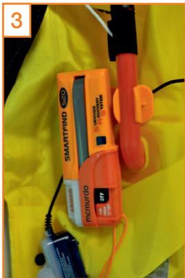
**Attaching the S20 to the lifejacket.** Open the left side of the lifejacket as worn, the side opposite the manual activation toggle. Attach the S20 low down on the oral tube as shown, between the base of the oral tube and whistle.
