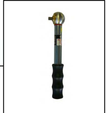
Calibrated Socket Driver (Tighten Cylinder)
