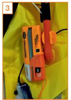
Attaching the S20 to the lifejacket. Open the left side of the lifejacket as worn, the side opposite the manual activation toggle. Attach the S20 low down on the oral tube as shown, between the base of the oral tube and whistle.
