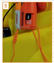
Attaching the lanyard. Using the remains of the orange lanyard (which is secured to the bottom of the lifejacket) tie loose end onto the white section of the S20 with a bowline. Ensure that there is plenty of slack in the line so the S20 is not pulled off the oral tube when the lifejacket is inflated. The purpose of this line is purely as a back-up in case the S20 is dislodged from the oral tube.
