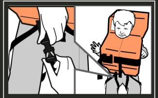
BRING CRUTCH STRAPS UP BETWEEN THE LEGS AND CONNECT BUCKLES BY PUSHING THE TWO BUCKLE PARTS TOGETHER.
