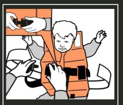
CONNECT BUCKLE BY PUSHING TWO PARTS FIRMLY TOGETHER
