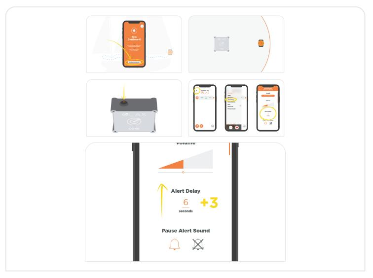
7. If a false alarm sounds again return to step 1 and increase the Alert Delay at step 5 in increments of 3 seconds.
