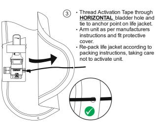
Activation Tape Threaded through hole in bladder.
