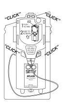
Position MyAIS Unit as shown. Ensure an audible "CLICK" is heard from each clip on the Strap Clip. The unit is now fixed and secure.
