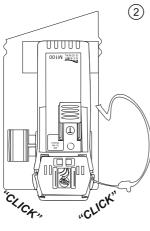
Position M100 unit as shown. Ensure an audible "CLICK" is heard from each clip on the Mounting Backet. The unit is now fixed and secure.
