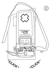
Position AISLink Unit as shown. Ensure an audible "CLICK" is heard from each clip on the Installation Backet. The unit is now fixed and secure.
