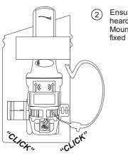
Ensure an audible "CLICK" is heard from each clip on the Mounting Backet. The unit is now fixed and secure.
