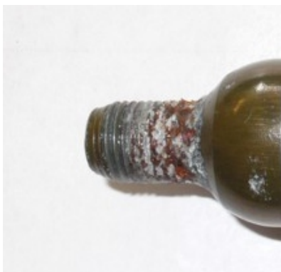
Cylinder showing red rust
