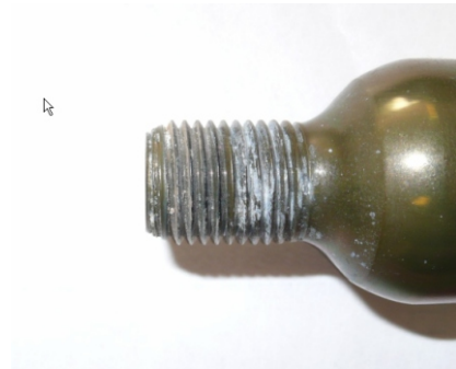
Cylinder showing white rust on thread
