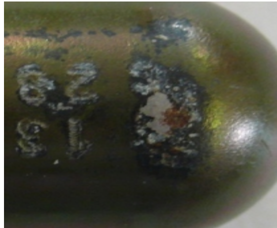
Not acceptable wear - Reject. DO NOT USE
