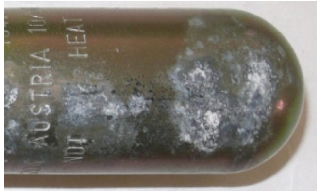
Not acceptable wear - Reject. DO NOT USE
