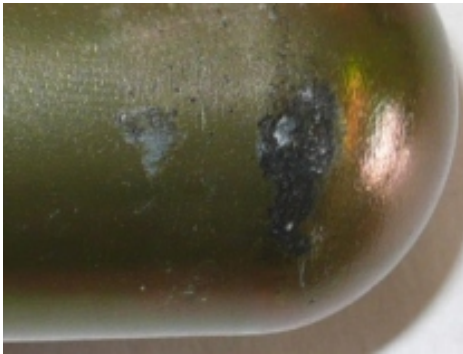
Acceptable wear - less than 1cm 2
