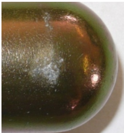
Acceptable wear - less than 1cm 2
