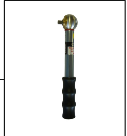
Calibrated Socket Driver (Tighten Cylinder)
