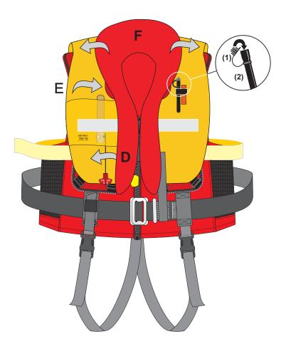
Ensure that the valve cap (1) is replaced on the inflation tube (2) after deflating the Lifejacket.
