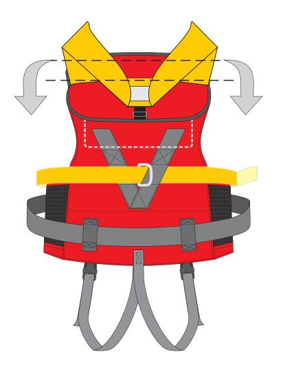
Turn the jacket over and fold the collar of the bladder down once, then pull the bladder cover over and fasten the velcro.
