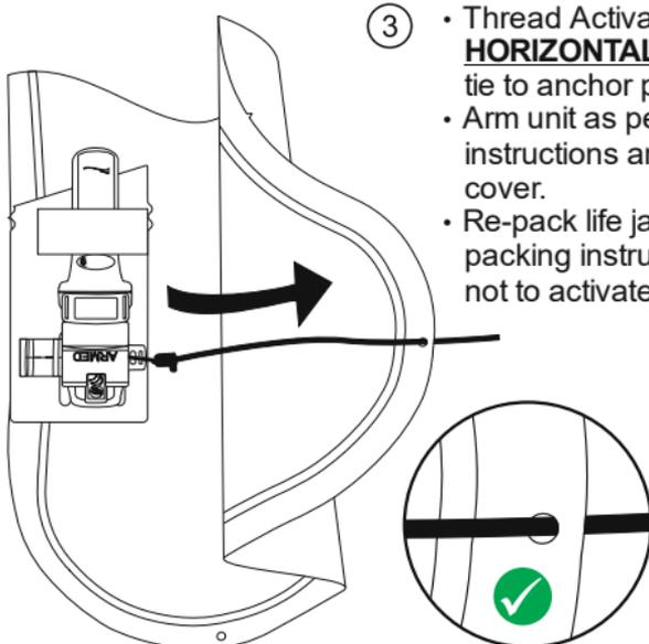
Activation Tape Threaded through hole in bladder.
